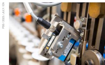
NEOSeam allows tube producers to re-purpose the «side trim», the laminate material which is normally cut off the printed material and then thrown away. The side-trim is used by NEOSeam to build-up the tube's sideseam, allowing the production of tubes which do not show any «white line» at the side seam area even after multiple uses.
